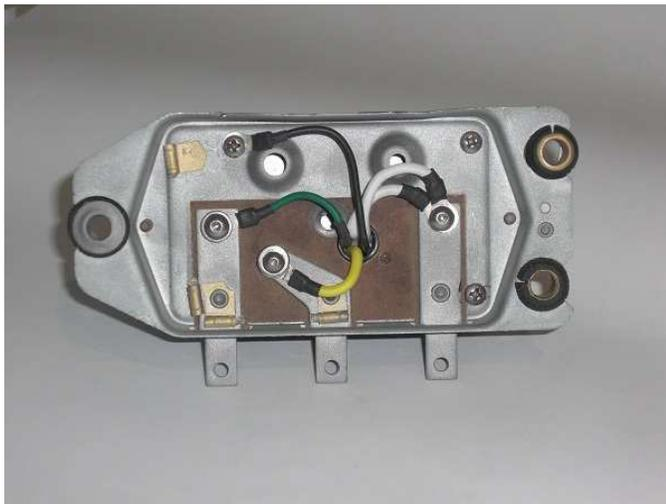
In this example, the wires exit from the bottom of the DRM, are fed through the base plate, and attach to the screw terminals. Use the existing holes where the relays were mounted, as they are already isolated from the (grounded) base. It's usually easier to attach the wires on the top.
