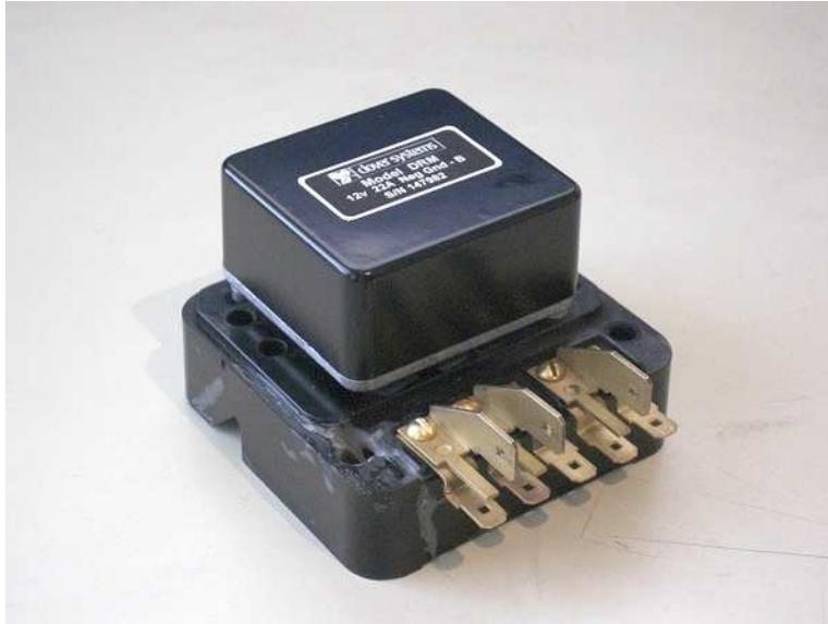
In this next example of mounting in a Delco CV regulator case (common on tractors), it's a tight fit, so it's necessary to mount it at an angle to provide clearance for the cover mounting screws.
