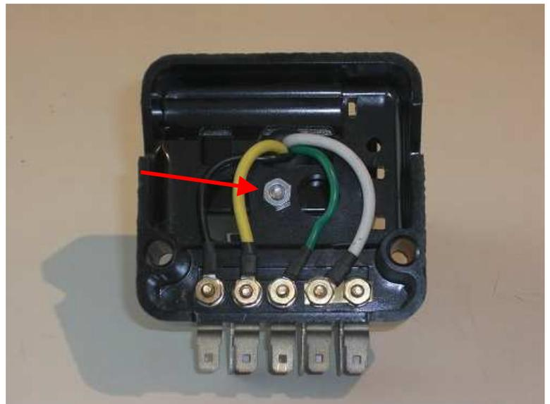
You can drill holes anywhere in the DRM cover for mounting, as long as your screws don't interfere with the circuitry.
