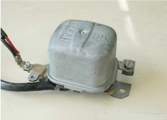
The problem with this mod is that due to the curved sides and the height of the Bosch regulator case, the DRM case will not quite fit inside. The solution is to remove the guts from the DRM and mount it to the Bosch regulator base. An additional problem is that the Bosch cover mounts with one screw in the center, which would have to go through the DRM to the base, which is not possible.
